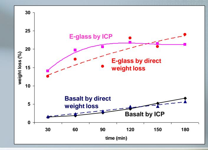
The resistance of basalt fibers to sulfuric acid is **4-5 times higher** than that of E-glass!
